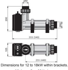
Minimum flow 90 l/min
